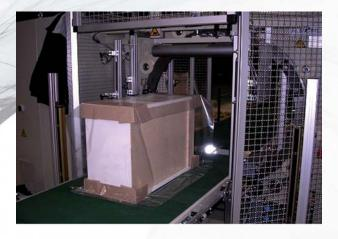
Fully automatic twist wrapping machine for all kinds of profiles and long products with high production capacity (TP = total pack – all sides wrapped).
